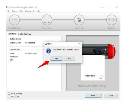
• The plotter will now automatically perform the calibration and report the correct laser offset for your device, which you need to confirm by clicking on "OK".
