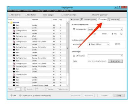
• Next, add your vinyl cutter by pressing the "Add" button (a Secabo S60 II is used in the example), select your model and click "Install".
